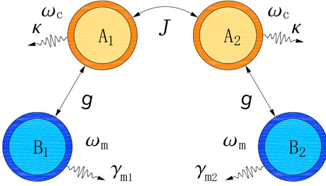
FIG. 1. Schematic representation of the system considered. Two phonon modes  $B_1$  and  $B_2$  with the same frequency  $\omega_m$  respectively interact with two photon modes  $A_1$  and  $A_2$ , which in turn are coupled via the photon tunneling.
